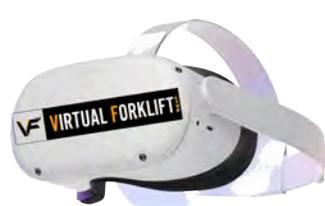
Customers that select the LIVE simulator training system, utilize the Oculus Pro 2 or 3 headset. This wireless option does not have the resolution of the HTC but still provides high quality simulation with the freedom of movement and multiple student interactions.
