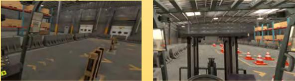
Once students get familiar with driving, they can practice pallet movements, pickup and put away in racking and cantilever racks and eventually move to box trailers, flatbed trailers and attachment specific training.
